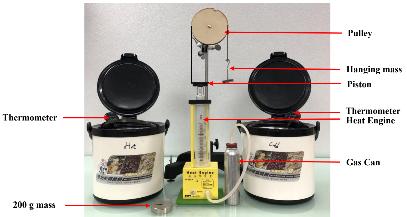
Fig. 9: Experimental setup of heat engine
