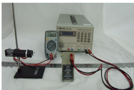
Fig. 8: Experimental setup for verifying the Stefan-Boltzmann law
