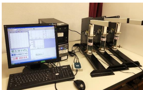
Fig. 10: Experimental setup of Isentropic compression
